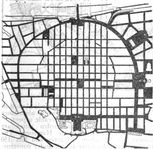
Great ground plan of Mannheim, Germany, a plan which with its outer horseshoe has proven highly satisfactory. It offers a solution of street replanning for American cities with their gridirons and has been followed in the proposed plans of Chicago and other cities.
